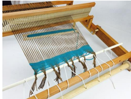
attach bundles to an apron rod
